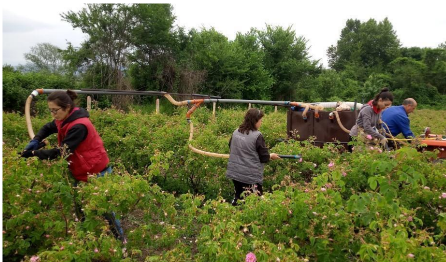
Figure 7.3. Experimental testing in field conditions of the three-row variant of the rose harvesting machine
