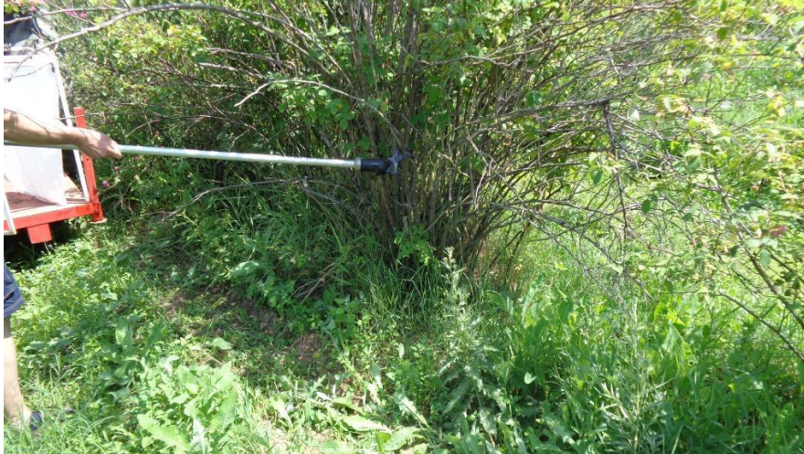
Figure 4.12. Testing the MMR variant for pneumatic selective pruning in rose plantations
